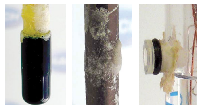
Innocuous crystallisation on storage cap, electrode shaft or refill opening
