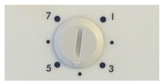
Such dials are simply numbered with the numbers not corresponding to any temperature. Having temperature monitored dial controlled unit it has been observed that the internal temperatures may be as cold as -38°C. This case study aimed to highlight the energy which could be easily saved by using a laboratory freezer at -20°C.
