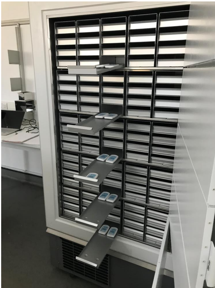
Figure 1. ULT freezer fully racked with temperature loggers in place.
