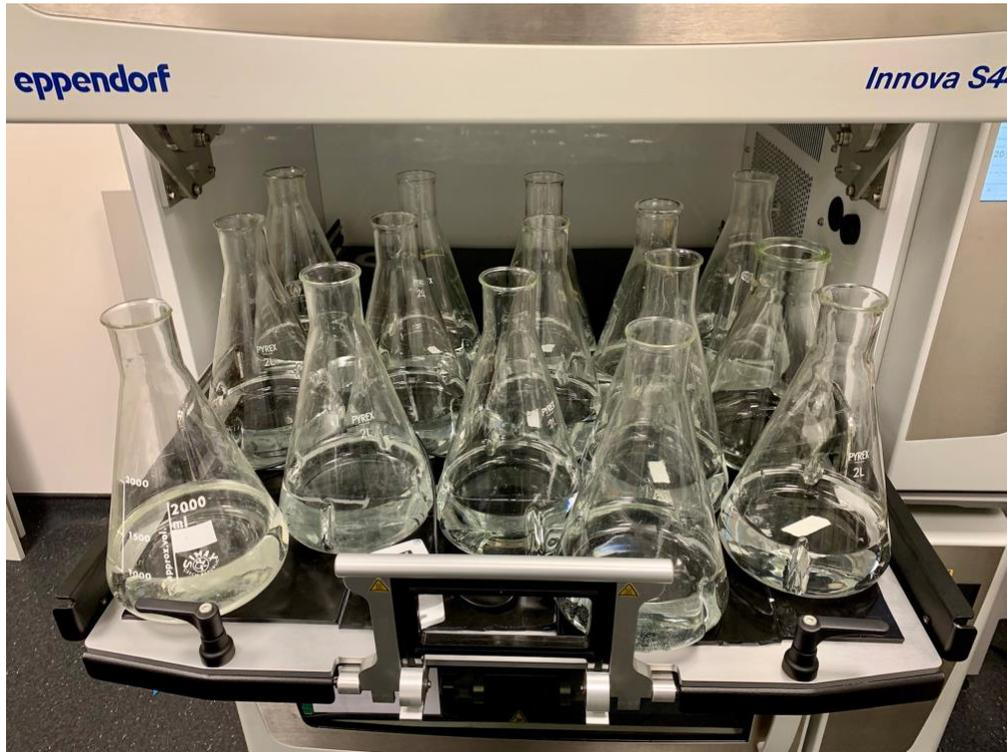
Figure 4. The Eppendorf S44i filled with 15 Erlenmeyer flasks.
