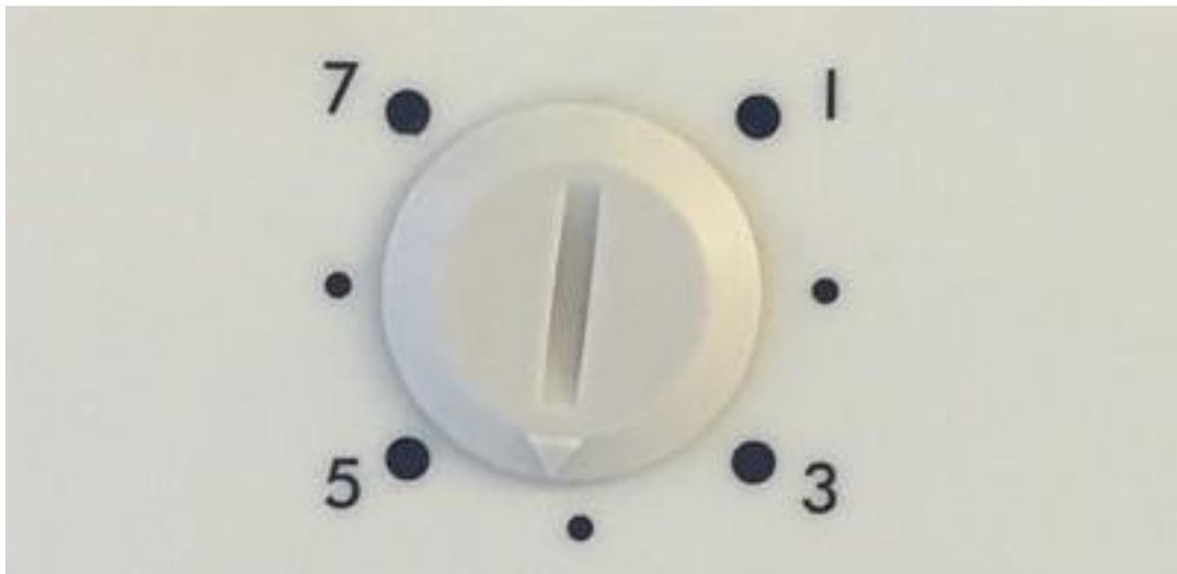
Such dials are simply numbered with the numbers not corresponding to any temperature. Having temperature monitored dial controlled unit it has been observed that the internal temperatures may be as cold as  $-38^{\circ}\text{C}$ . This case study aimed to highlight the energy which could be easily saved by using a laboratory freezer at  $-20^{\circ}\text{C}$ .
